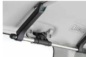
Attach the frame of the rod holder to the fixed grab handle adaptor
