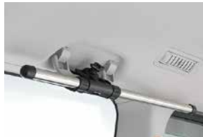
Insert the assist pipe through the grab handle adaptor
