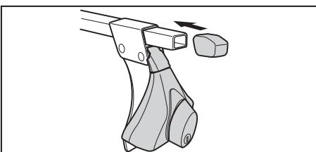
**14** Attach the end caps (included in the bar set) to both sides of the bar.
