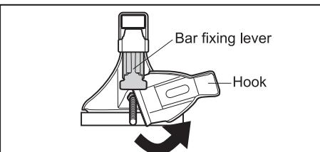
**15** Unlock using the key, remove the knob, cover, and the hook from the roof.
