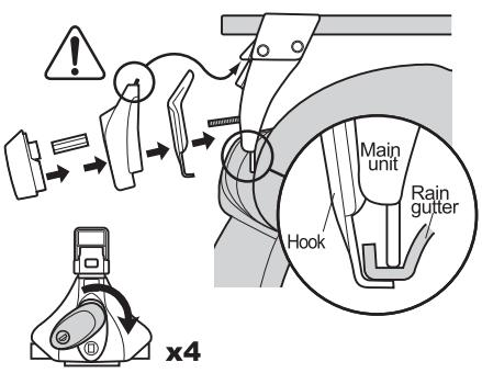
**10** Place the stay main unit on the rain gutter and secure the hook below the rain gutter. Pass the cover and the high nut accordingly through the installation bolt, and temporarily fix with the knob.
