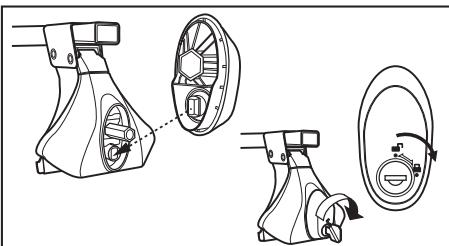
**13** Securely insert the knob key end into the cover lock hole to lock the key. After locking the key, check that the key does not come off by pulling the knob.
