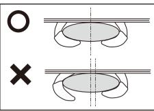
2 Make sure that the memory mount hooks are symmetrically positioned. If the center between hooks matches the base rack center, they are correctly positioned.
