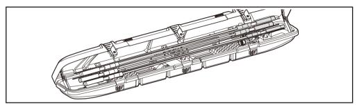
3 When placing multiple rods, alternate the direction of each rod's grip / tip.
