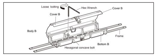
**3** Open Cover B. Align the nut on the frame edge with the hole on Bottom B that is proximate to the center. Loosely bolt all of four nut portions with the hexagonal concave bolt.
