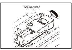
2 Close the lever. Turn the adjuster knob as the arrow indicates (or clockwise) to align the centers of both books and the base rack
