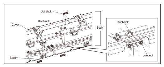
**8** Align the hole on the flange portion of Bottom A and C with the convex shape on the joint nut center. Fixate from the inside using the knob bolt.
