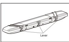
**3** Check that the three levers are securely closed, and the keys are locked.
