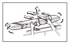
1 Shake the rod box in all directions, right and left, backward and forward, and up and down, to look for any rattling caused by improper installation. If you still hear or feel rattling, go back to Section 4 "Installation of the Rod Box" on page 7, and repeat the tightening procedures to re-tighten the two installation positions.
