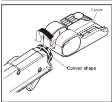
3 Open the lever, and rotate the adjuster knob to the direction indicated by the arrow (counter clockwise) by about 5 turns to make the hook space narrower. Confirm that the base bar center matches the center between hooks, close the lever to securely tighten. If the lever is loose, rotate the adjuster knob more. If the lever is too tight, reverse the direction of the adjuster knob and securely tighten.
