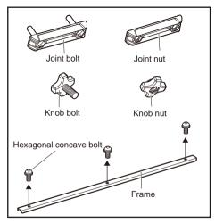
**2** Remove all of the joint bolts, the joint nuts, the knob bolts and the knob nuts from the cardboard.
