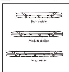
The length of this product can be adjusted at three levels according to your longest rod.
