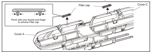
**5** Remove the filler caps on Cover A and C as necessary, depending on your position.
