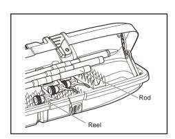
**2** Place your rods with their reels attached. Adjust the loading positions of the rods.
