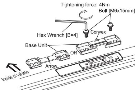
Place the base unit, included the base rack stay on the base plate and securely tightened the bolts [M6x15] alternately. Confirm the direction of the base unit.
