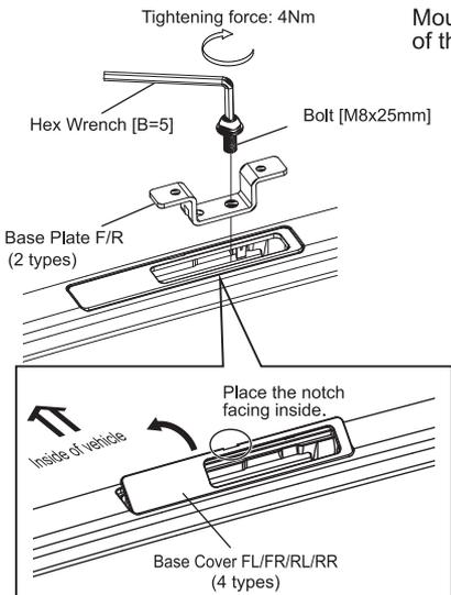
Mount the base cover, place the base plate on the mounting area of the vehicle, and firmly tighten the bolt [M8x25].
