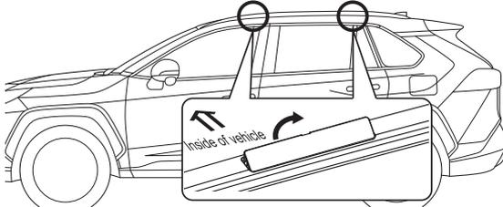
Remove the carrier installation cover located on the roof rail of the vehicle.
