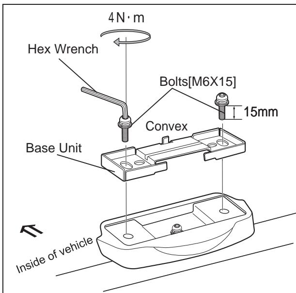
1 Place the base unit on the installed cushion base/base bracket. Then using the Hex wrench (included), tighten while alternating between the right and left bolts (short) [M6x15] (supplied with the carrier) until the bolts are firmly tightened.
