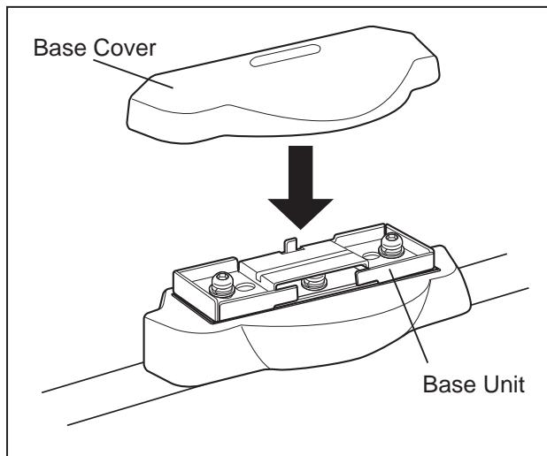
After removing the stay and the bar, leaving only the base unit on the vehicle, apply the base cover to the base unit.
