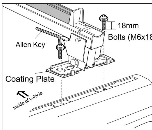
**1** Place the coating plate and carrier on the nut plate that you inserted into the genuine roof rail, and using the Allen key, tighten alternately the right and left bolts [M6x18].
