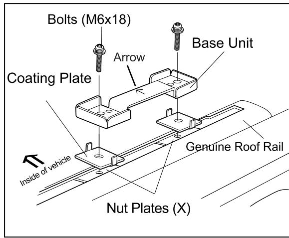
**1** Place the coating plate and base unit on the nut plate that you inserted into the genuine roof rail, insert a bolt [M6x18mm] from the outside, and loosely screw them together.
