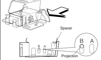
Place the bolts through the carrier, rubber spacer, front hook and rear hook in this order and loosely screw the bolts. Verify the direction of the Tnut in doing this. Repeat this procedure for the opposite end.
