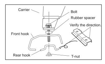
Place the bolts through the carrier, rubber spacer, front hook and rear hook in this order and loosely screw the bolts. Verify the direction of the T-nut in doing this.
