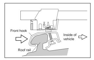
Slide the front hook so that it is pressed onto the roof rail.
