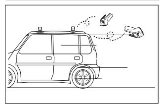
Tighten bolts alternately using the attached allen key and fixate the stay onto the roof rail.
