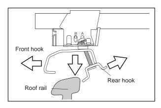
Insert the bar into the assembled stay. Open the front hook and rear hook manually, and place them on the roof rail.
