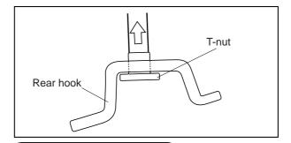
Insert the T-nut projection into the hole of the rear hook.
