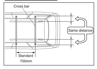
Lay the cross bars vertically against the roof bars.
