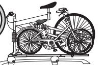
Do not load anything other than a bicycle or load more than one bicycle onto a single attachment system.
