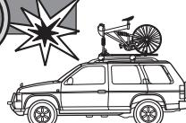
Before driving the vehicle, always check the vehicle's overall height, including the bicycle loaded on the roof of your vehicle, and remind yourself to be aware of low-clearance parking garage, tunnels and other structures.
