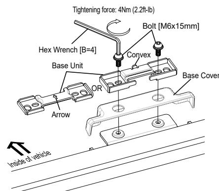
Cover the mounted base plate with the base cover, place the base unit included in the rack unit on it, and securely tighten the bolts [M6x15] alternately. Confirm the direction of the base unit.
