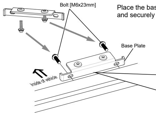
Place the base plate from the inner side of the rail to the location and securely tighten the bolts [M6x23] alternately.
