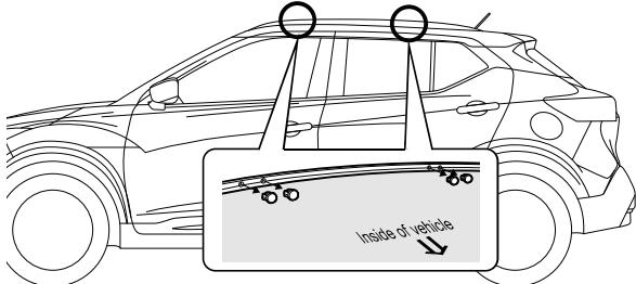
Remove the caps that are located inside the roof rail. (8 pieces in total for right and left)
