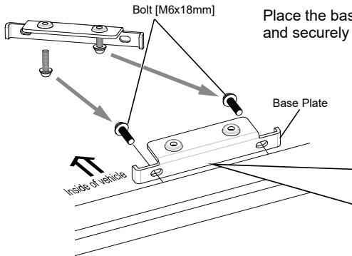
Place the base plate from the inner side of the rail to the location and securely tighten the bolts [M6x18] alternately.
