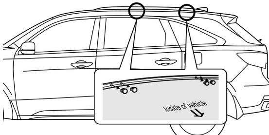
Remove the caps that are located inside the roof rail. (8 pieces in total for right and left)
