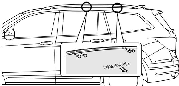
Remove the caps that are located inside the roof rail. (8 pieces in total for right and left)
