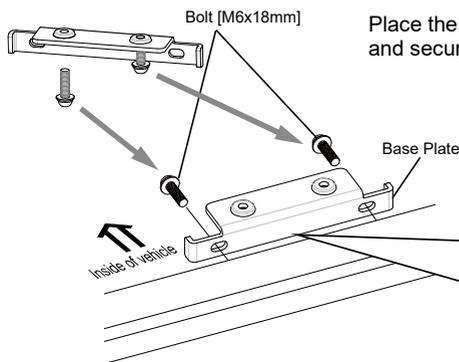
Place the base plate from the inner side of the rail to the location and securely tighten the bolts [M6x18] alternately.
