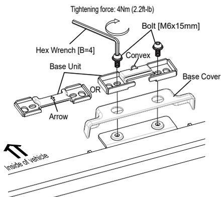
Cover the mounted base plate with the base cover, place the base unit included in the rack unit on it, and securely tighten the bolts [M6x15] alternately.
