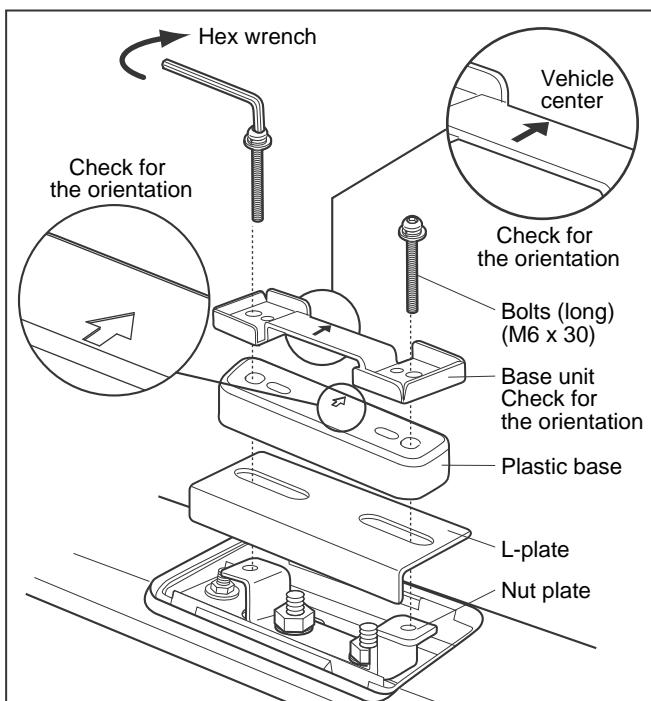
**1** Fix the base unit to the nut plate using the bolts (short) (M6 x 15) (the base unit and the bolts are supplied with IN-XR). In this case, the L-plate must be placed underneath the base unit.
