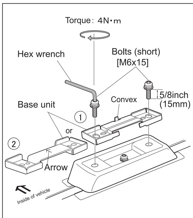
**1** Place the base unit on the installed cushion base/base bracket, and using the Hex wrench, tighten alternately the right and left bolts (short) [M6 x 15] until the bolts are firmly tightened.
