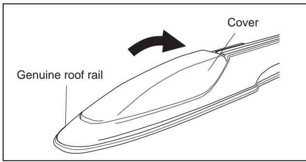
**3** Open the cover on the front of the roof rail.
