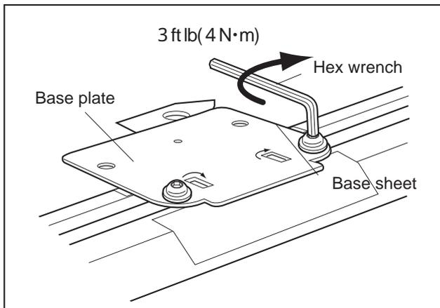
**5** While slightly raising the base plate, slide it to the position where the base sheet is attached, and tighten it with the included hex wrench until it is firmly fixed.
