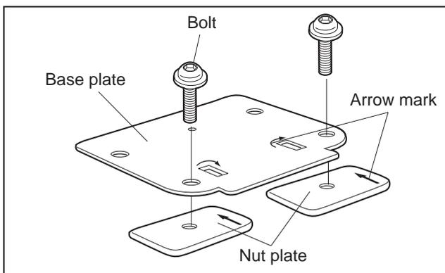
**2** Loosely screw together the nut plate and the base plate using the bolt [M6x15mm].
