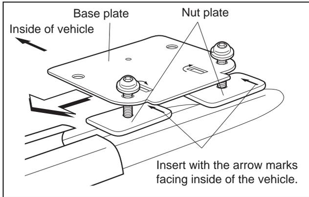
**4** From the front of the roof rail, slide the loosely assembled base plate and insert the nut plate into the groove of the roof rail as illustrated. Be sure to insert the nut plate with the arrow marks facing the inside of the vehicle.
