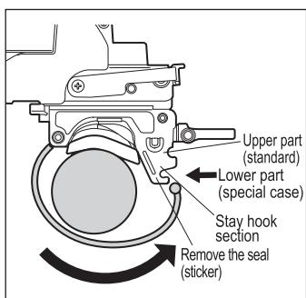
If the multi strap is extended to its maximum length yet it still does not reach, remove the seal and hook the strap onto the lower level of the hook section.
