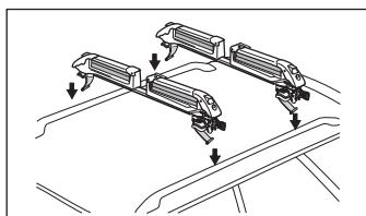
⑥ Align the depressed part of the base section of the stay with the center of the roof rail, and place the carrier on the rails.
