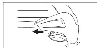
Insert the carrier cover firmly as far as it will go. If it is not inserted firmly, the carrier cover will rattle. If the carrier cover rattles, insert the cover again correctly.
