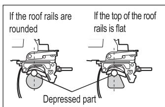
⑦ Adjust the position of the carrier so that the bindings can rest between the front and back carriers.
