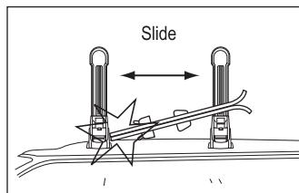
⑨ When you have decided on the installation position, mark the positions using the tape.
