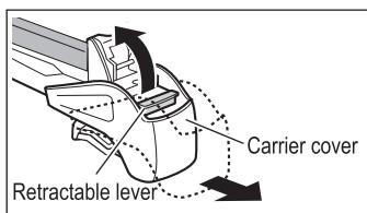
When the cover is removed, the carrier's stay is exposed.
