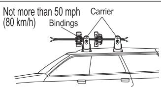
If the ski or snowboard bindings do not fit between the front and back carriers, arrange so that one of the bindings is to the front side of the front carrier.
