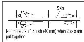
If the ski or snowboard bindings do not fit between the front and back carriers, arrange so that one of the bindings is to the front side of the front carrier.
