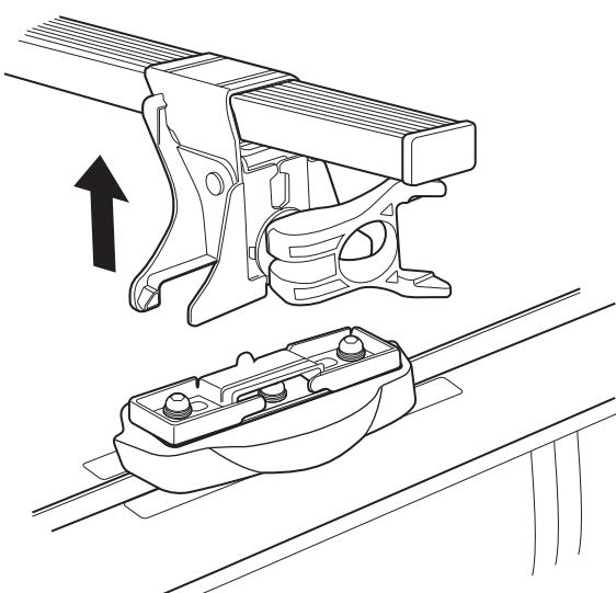
**2** EN: With the lever facing sideways, lift the lever up while pushing the lever center to remove from the vehicle.
