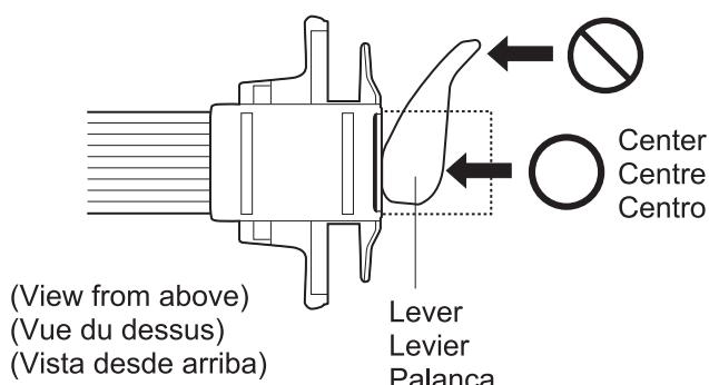
**Note** Placing on the base unit while pressing the center of the lever, makes the hook open completely, therefore making it easy to insert.
