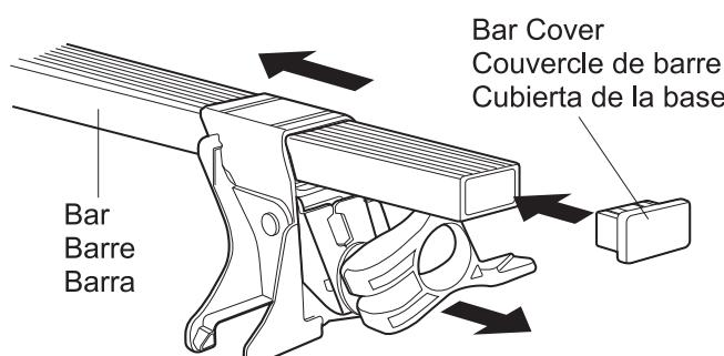
**1** EN: Unlock and remove the cover.
