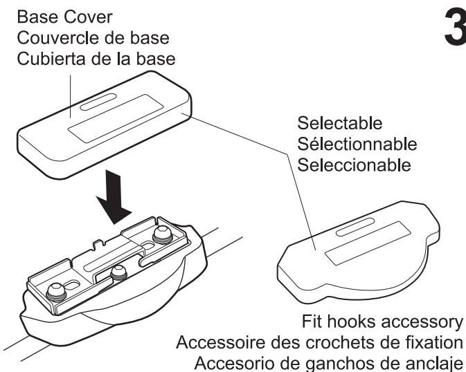
**3** EN: After removing the stay and bar, only the base unit remains on the vehicle. Attach the base cover to the base unit.
