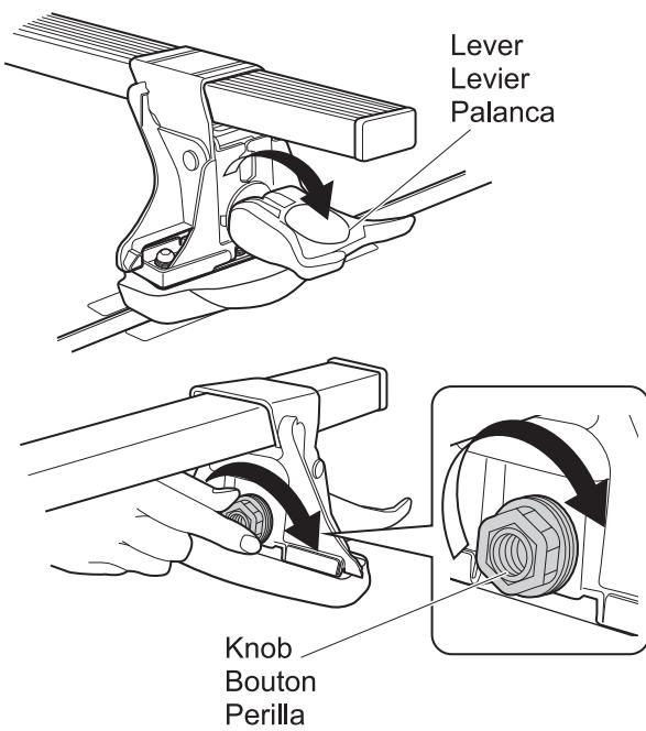
**8** EN: To secure the initial fit, while pushing the lever, tighten the adjustment knob located on the back side until it stops.
