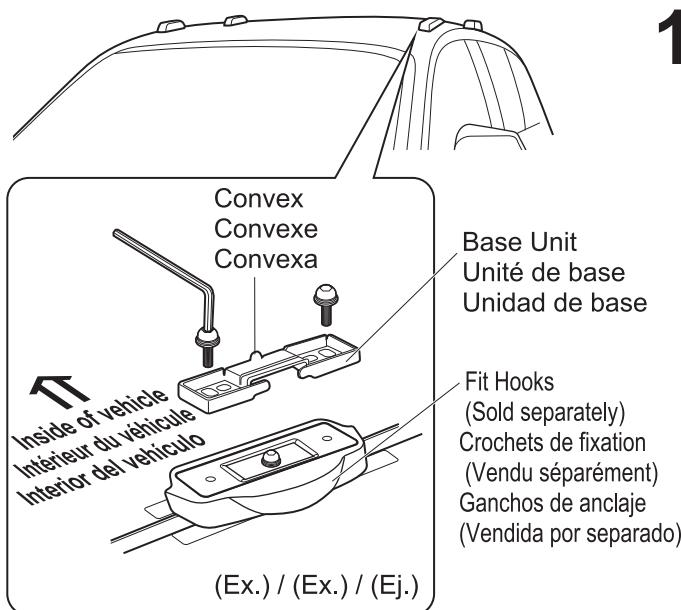
**1** EN: Mount the base unit in a way that the convex section is on the inner side of the vehicle. Mount the base unit according to the vehicle-specific installation procedure listed in the mounting hook installation instructions.
