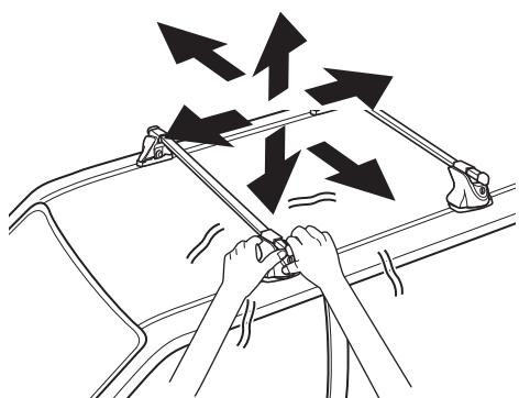
**1** EN: Shake the rack in all directions to make sure that it is securely fastened, if loose adjust the knob accordingly.
