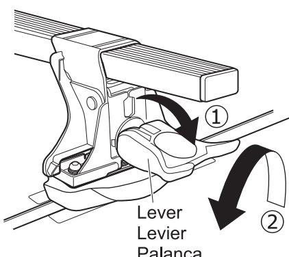
**1** EN: ① Open the lever ② Rotate the lever 90 degrees
