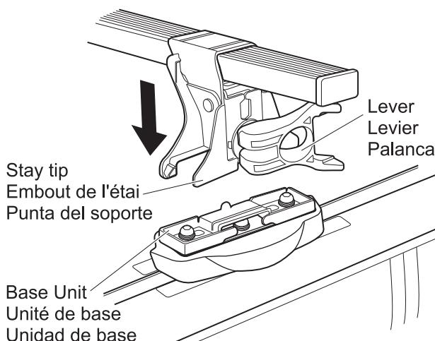
**1** EN: With the lever facing sideways, place it on the base unit while pressing the center of the lever.
