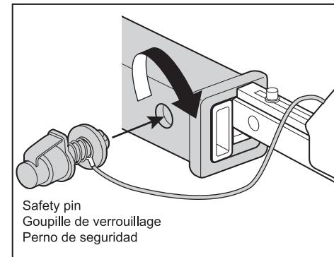
**5** EN: Insert the safety pin through the base hole groove, and turn **90°**.
