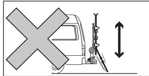
● Load snowboard upside down if snowboard is not long enough so tail-end of snowboard is closer than 4" (100mm) to the lower horizontal bar of the attachment.
