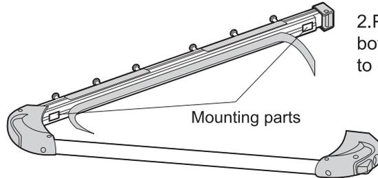
3. Insert bolt in square hole from back of hitch base, and attach washer, spring washer and hexagon socket nut using with hex wrench. (Reference torque 5Nm) Attach lower attachment as well.
