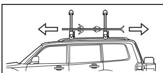
When loading short ski/snowboards on to the carrier, please check to see if the carrier is properly adjusted for the short ski / snowboard.
