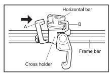
**1** Loosen the levers in 4 places of the cross holder to move A downward.
