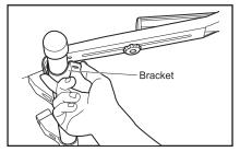
**3** Mount the bracket from below, and temporarily fix in place.
