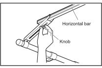
**4** Raise the horizontal bar as high as possible while having the adjuster touch the horizontal bar so that the bar becomes horizontal, and temporarily fix the knob in place.
