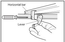
**2** Raise A to insert into the groove of the horizontal bar, and fasten the lever.
