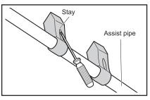
When the pipe touches the interior or when a hand cannot be inserted in the space between the headlining and the pipe due to lack of room, install the stay upside down or insert Spacer 1 and tighten the screw.
