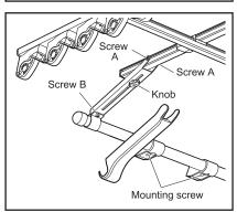
**3** To adjust the horizontal bar height to make it as high as possible using the adjuster, paste the pad to the place contacting the lining, and tighten all screws.
