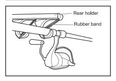
Push the rubber bands in the order of front and rear to hook to the bottom of the hook.
