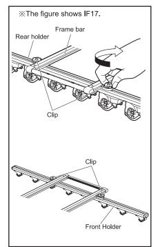
**3** Fix the front and rear holders with clips from outside the frame bars.
