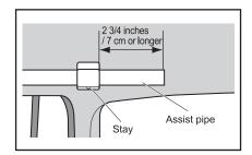
**3** Put the assist pipe through the stay from the side and temporarily fix the stay with the pipe protruding at least 2 3/4 inches or 7 cm. Temporarily tighten the mounting screw to prevent the pipe from rattling but allowing the pipe to slide backward and forward.
