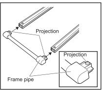
**2** Match the projection of the fame cap to the hole of the frame bar to insert.
