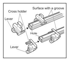
**1** Fit 2 cross holders in the frame bars by making the levers stay outside the frame bars.
