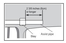
3. Put the assist pipe through the stay from the side and temporarily fix the stay with the pipe protruding at least 2 3/8 inches or 6cm. Temporarily tighten the mounting screw to prevent the pipe from rattling but allowing the pipe to slide backward and forward.
