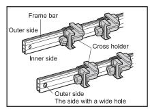
1. Insert a frame bar into the 2 cross holders facing the same direction.
