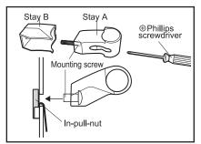
③Insert the included mounting screw into Stay A, and put Stay A into Stay B. To temporarily hold the stay on to the vehicle body, insert the mounting screw into the in-pull nut, then tighen the mounting screw with Phillps screwdriver.
