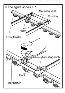
Attach the front and rear holders to the frame bar using the hooks and the mounting knobs.
