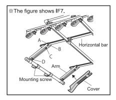
3. Adjust the height of the horizontal bar using the adjuster (see Page 4), and tighten screw A, B, C, and D and mounting screws.
