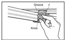
2. Lift F to insert the groove of the horizontal, and tighten the knob.
