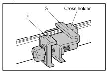
1. Loosen the cross holder knobs in 4 places, and slide F downward. Adjust the front and the rear of the cross holder, and insert G into the groove of the horizontal bar.
